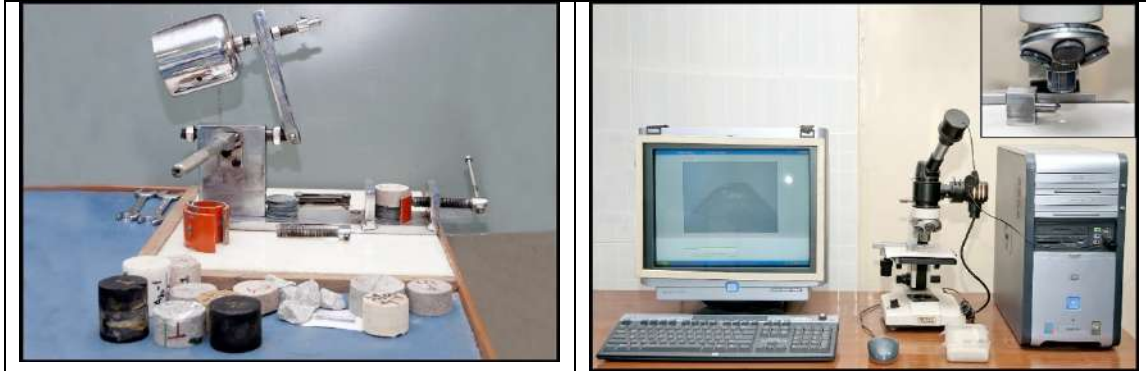
Fig.2: Test setup for Cerchar Abrasivity Index (CAI)
