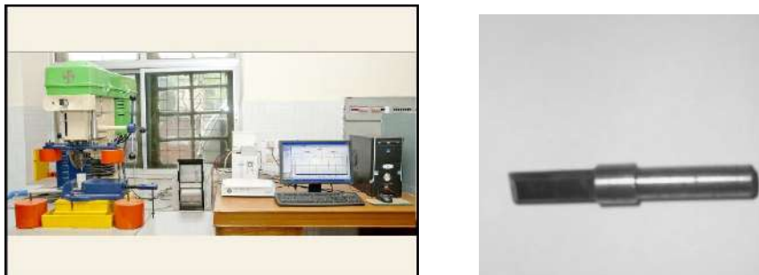
Fig.5: Test setup for Siever’s J value determination
