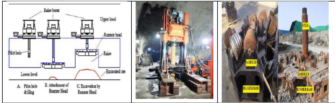
Fig.18 – Deployment of raise boring machine
