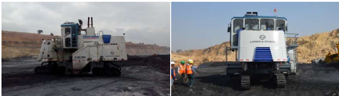
Figure14 : Surface Miner under operation at Jayant mine of NCL
