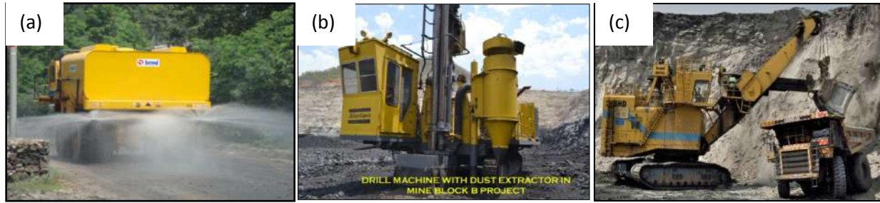
Figure 8: Air pollution control measures taken by NCL: (a) Water sprinkler for dust suppression at haul roads, (b) Drill machine with dust extraction system, (c) HEMMs with dust proof cabin
