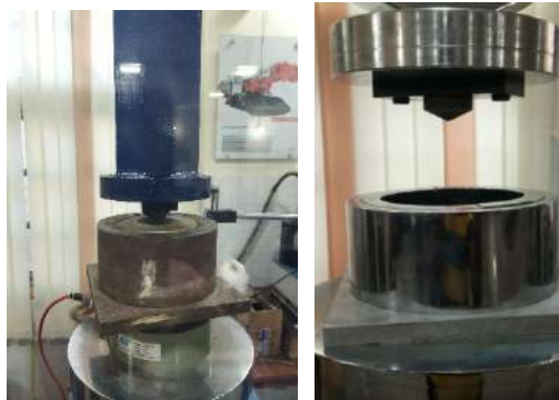
Fig.9: Punch penetration cell with indenter in PPI Test
